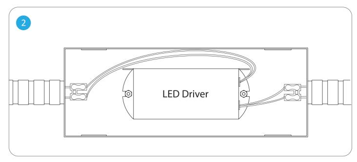
Using the provided DC cable & connectors, connect the wires inside the transformer enclosure as illustrated in the Wiring Diagram below.
