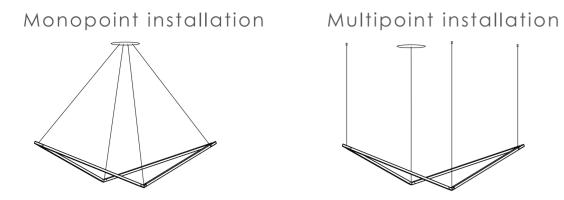
There are two ways to mount the Z-Bar pendant bird, a monopoint installation or a multipoint installation. For monopoint installation, proceed to step 2. For multipoint, see below.
