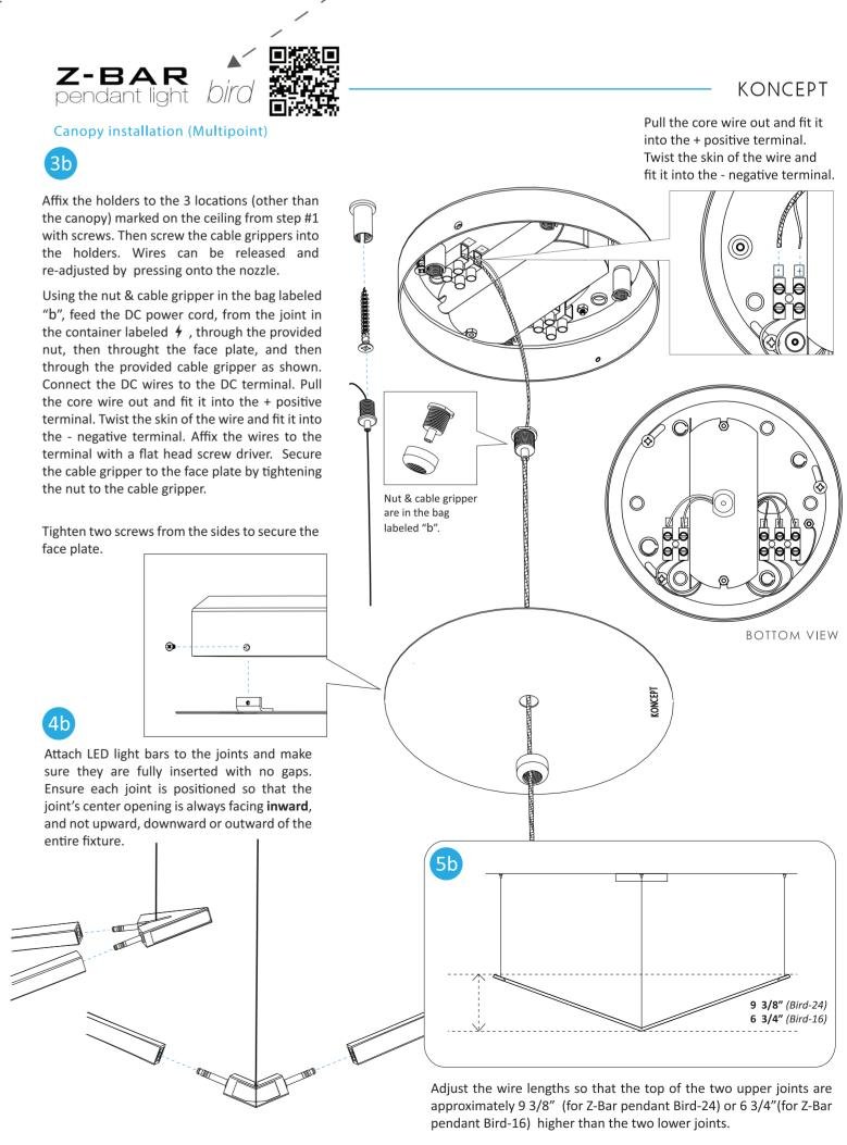
Wires can be released and re-adjusted by pressing in the cable
