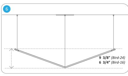
Adjust the wire lengths so that the top of the two upper joints are about 9 3/8" (for Z-Bar pendant Bird-24) or 6 3/4"(for Z-Bar pendant Bird-16) higher than the two lower joints.
