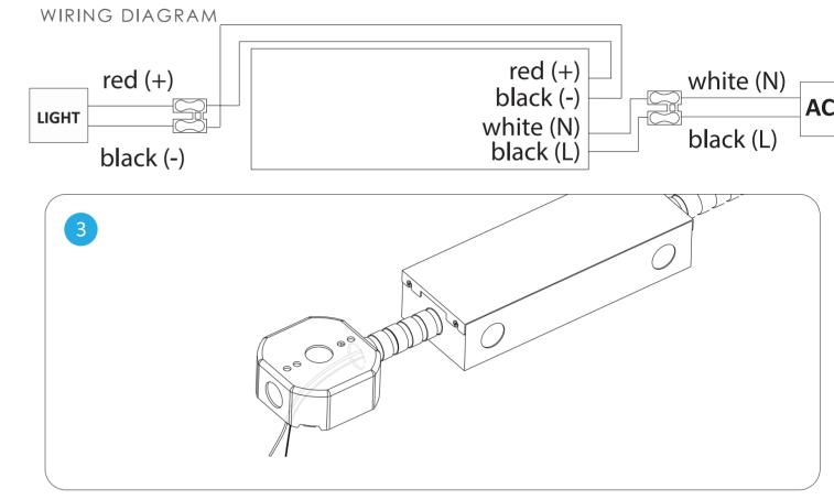
Feed the Red and Black DC wires through the conduit into the junction box (conduit and junction box not provided). Affix the transformer enclosure and junction box properly inside the ceiling, with an opening allowing access to the junction box.
