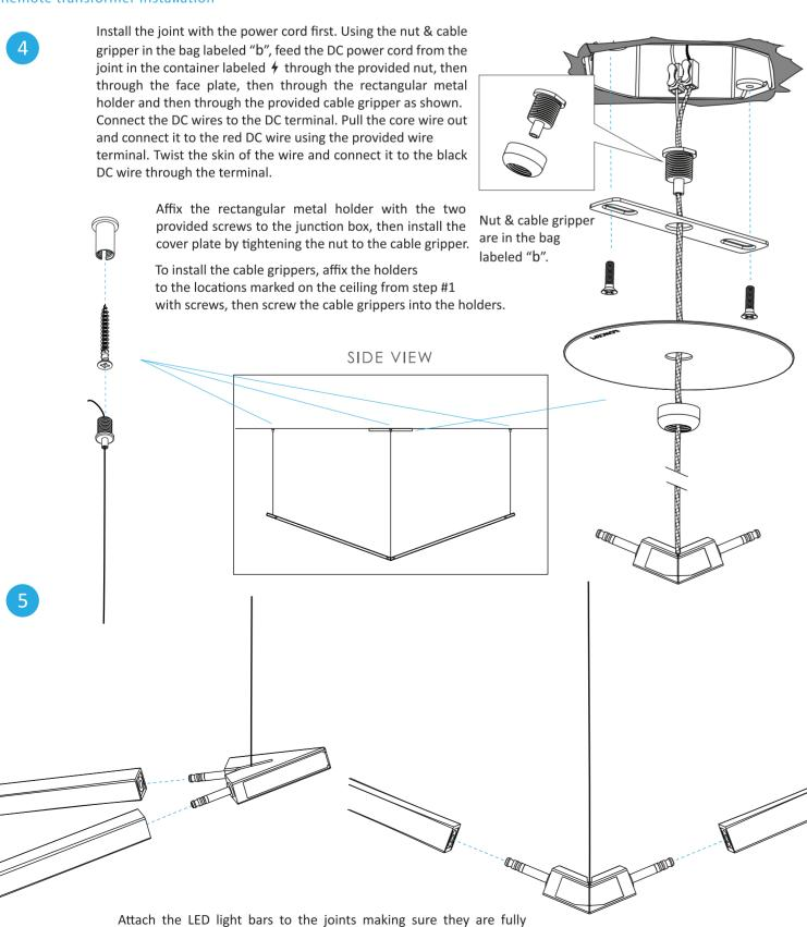
inserted with no gaps between the light bars and the joints. Ensure every joint is positioned so that its center opening is always facing
