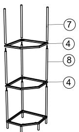
1.Place final frame 4 onto unit and screw ball ends (3) into short poles (7).
