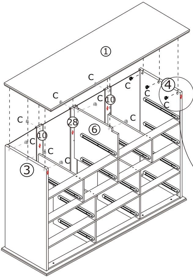
Cover board 1 to the top, add cam lock(C) into board 3,10,28 ,6,4 and turn clockwise to tighten as shown.
