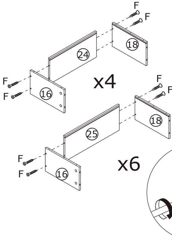
Fix board 24 to board 16 and 18 with screw(F), insert bottom board 26 along grooveas shown. Fix board 25 to board 16 and 18 with screw(F), insert bottom board 27 along grooveas shown.
