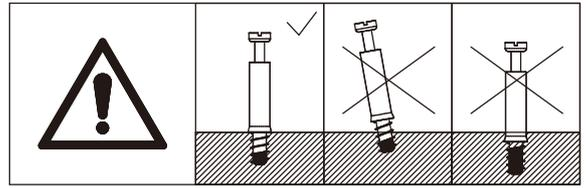
Screw eccentric rod(A) into board 2 as shown.
