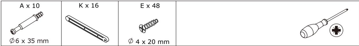
Fix rail(K) to board 3 and 4 with screw(E), and screw eccentric rod(A) into with a screwdriver as shown.
