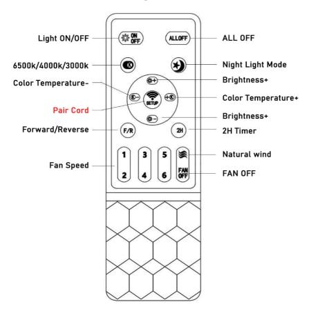
Battery Information: 2pcs AAA batteries needed If not used for a long time, remove the battery.
