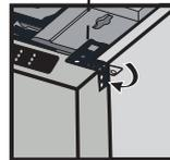
If necessary (according to counter top board material), bend sides of mounting brackets.
