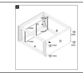
**Step4:** Fix frame Metal (E) on frame (A&B) using (HW2) Phillips screws. Meanwhile, install 4 Wheels into plate (D)
