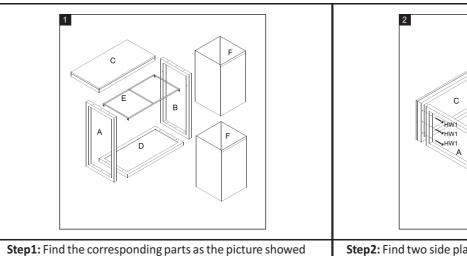
**Step2:** Find two side plate (A&B) and fix them to plate (C) and (D) respectively, using (HW1)Hex socket screws
