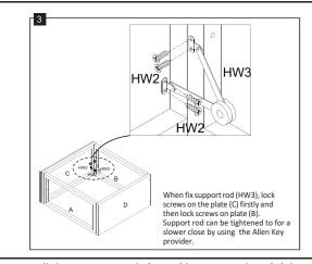
**Step3:** Install the support rods (HW3) between plate (B) & plate (C) using (HW2) phillips screws
