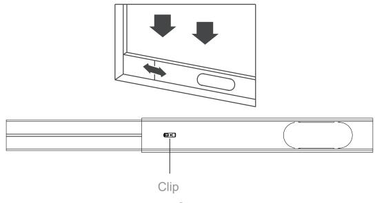
Usually Portable air conditioner needs to be equipped with sliding windows. We put two sealing plates in the packaging box of the machine, and the size range after connection is **94cm-127.5cm**(37in-50.20in). We also have two spare parts, one short(40cm=15.75in) and one long(67.5cm=26.57in)with"Clip".
