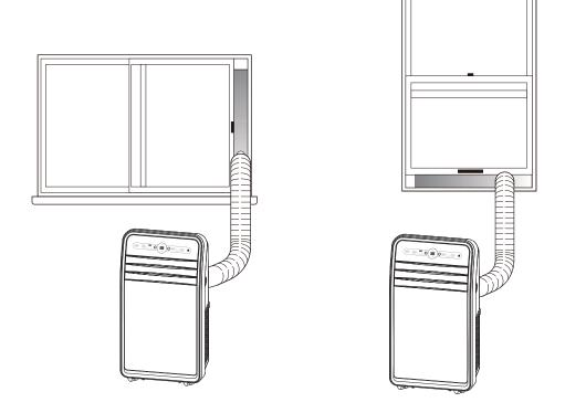
**Note:**For optimum performance, make sure the venting hose is not twisted and is free of kinks. For better efficiency, shorten the hose by squeezing its sections together.
