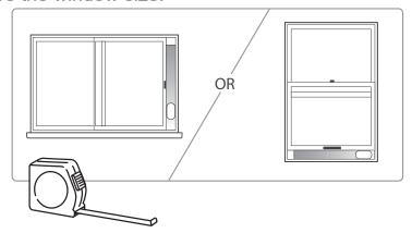
3.Install the window sealing plate in the window opening, adjusting the length to fit the window opening and securing it with "Clip" (provided). **Note:** The window sealing kit works with sliding windows.
