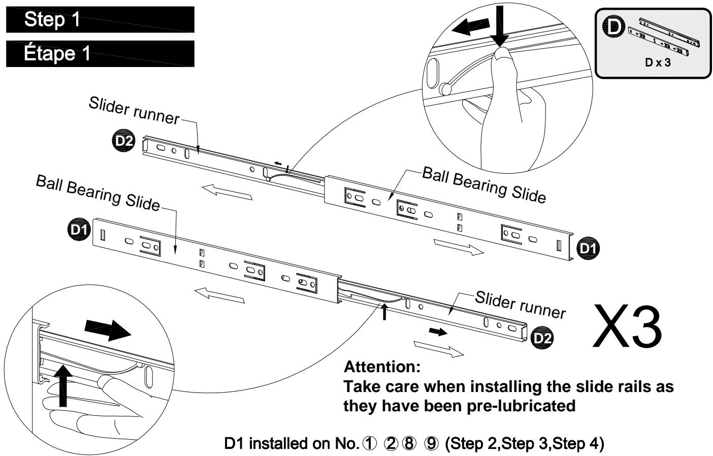
D1 installed on No. ① ② ⑧ ⑨ (Step 2, Step 3, Step 4)
