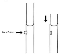
To fold the chair flat, press in on the lock button on each leg.
