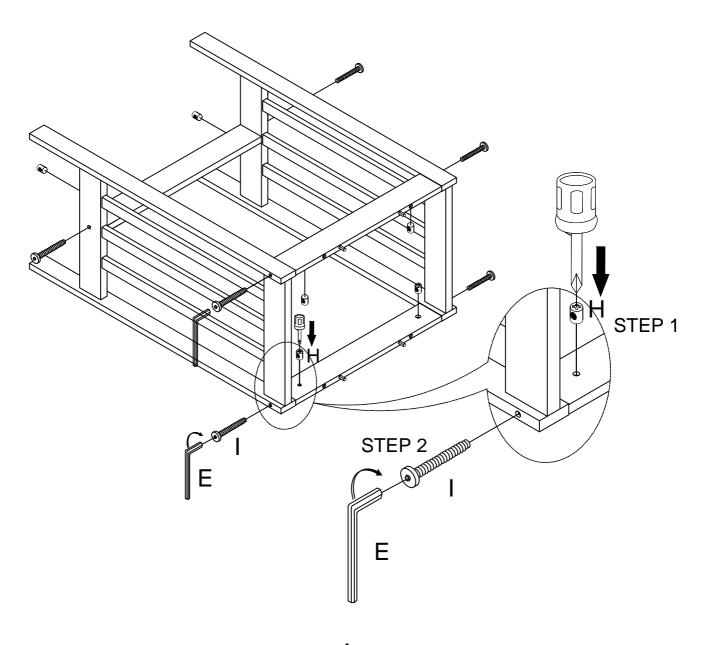
Place top upside down on a clean cloth for table base assembly. Place table base to the table top with alignment of wood dowels at two inner holes. Insert bolts (I) to the holes at cross bar and turn clock wise with allen wrench (E) until tight.
