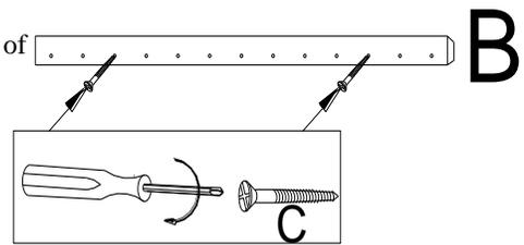
**It is recommended that the cleat (B) be securely screwed into the studs for stability.**
