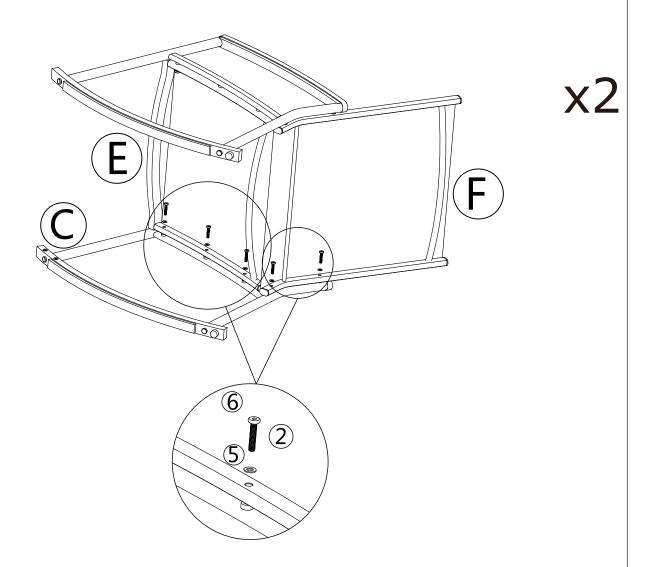
Fix part F and part C with two M6x30mm Screws (2) and (5) Flat Washers.Use (7) Allen key. **DO NOT YET TIGHTEN.**
