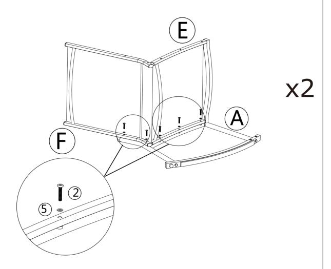
Fix part F with part A with two M6x30mm Screws (2) and (5) Flat Washers.Use (7) Allen key. **DO NOT YET TIGHTEN.**
