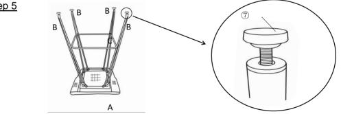
Install the Leveller(①) into the bottom of the Chair Leg(B), tighten by turning the Leveller clockwise.
