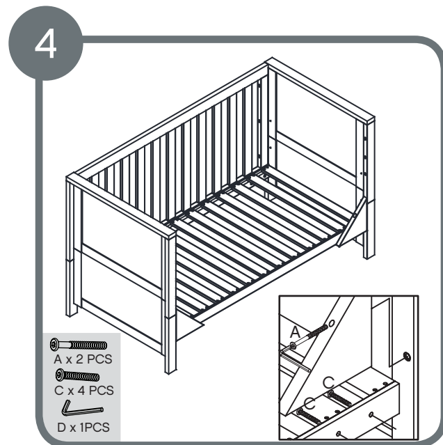
Assemble triangle braces support using 2 x A bolts and 4 x C bolts
