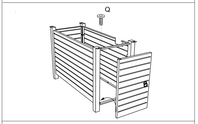
2. Hang the bottom (G) of the door plate on the round bracket. Top with 1PC screw(Q)lock.
