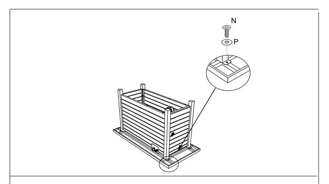
3.Attach the assemble base to the bottom of top using 4pcs of screws (N), and 4pcs M6 washers(P), make sure the panel (K) faces the valve stem.
