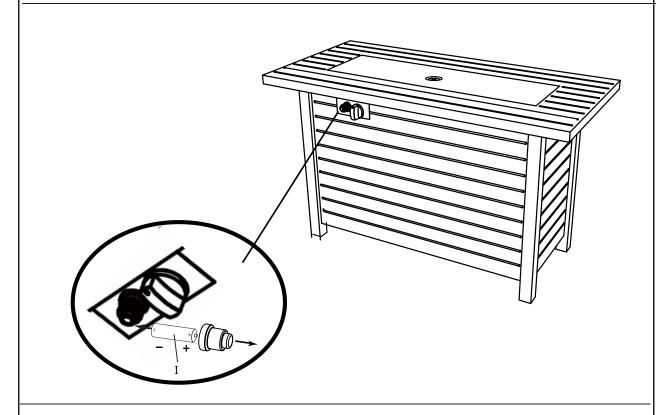
6.Remove the rubber cap on the electronic igniter by unscrewing and slide battery (I) into the battery slot. Make sure the positive side of the battery faces outwards. Screw the electronic igniter cap over the battery tightly.
