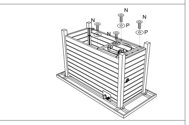
4. Connect the tank holder/base (I) With table Lets(A/B/C) by 4pcs screws (N) and 4pcs M6 washers(P). Tighten all screws.
