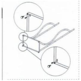
2. 4 nets are fixed on the left and right supports from bottom to top with screws and nuts;
