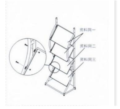
3、 The advertising board is fixed on the left and right brackets with screws and nuts;
