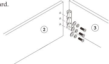
Before tightening the bolts, please ensure the bed frame is square.
