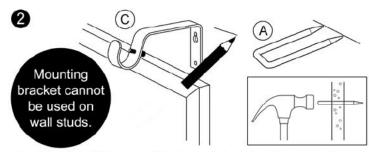
Use bracket (C) as a guide to mark location for mounting bracket (B). Use hammer to tap pilot hole tool (A) into wall. If you feel that the tool has contacted a stud, gently remove tool from the wall using pliers or a screwdriver if needed.
