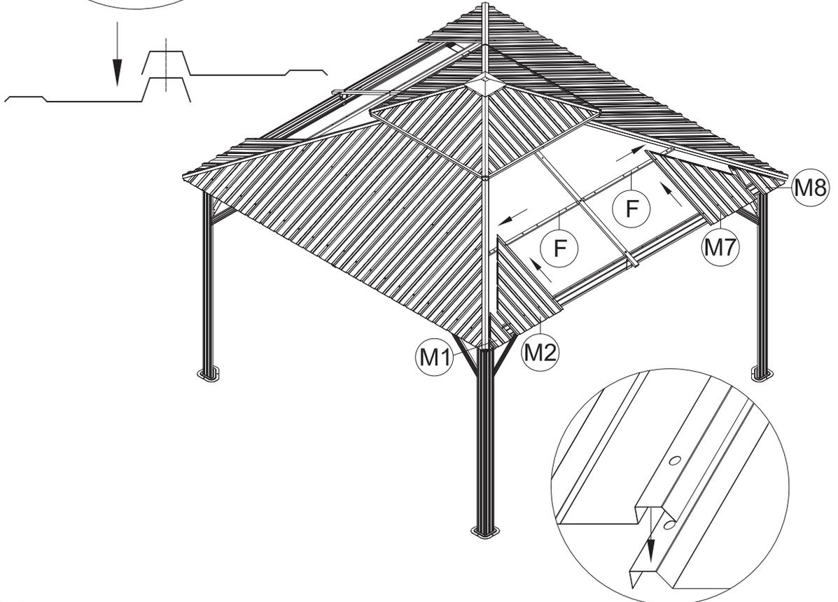
(2) Insert Part #M8 and Part #M7 into the frame.
