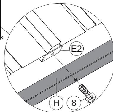
(3) Attach Part #H to Part #E2, securing with Bolt #8.
