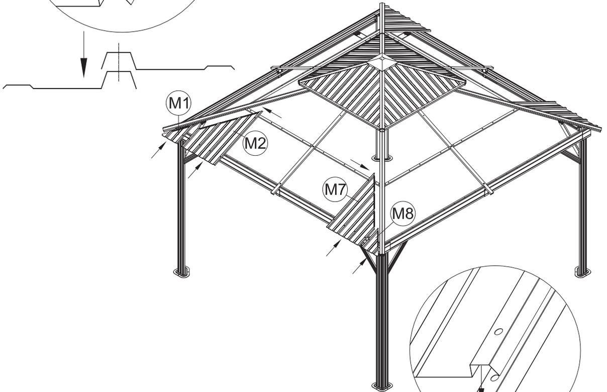
(2) Insert Part #M8 and Part #M7 into the frame.
