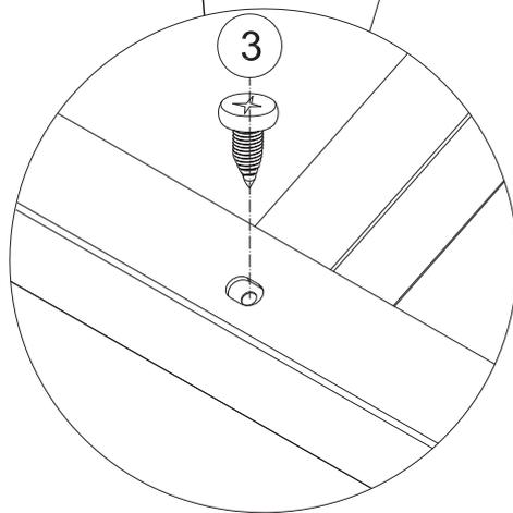
(1) Attach roof panels to finishing bars with 2 Self-tapping Screws #3.
