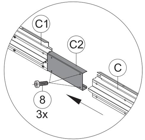
(2) Insert the other side of Part #C2 into Part #C and secure with 3 Bolts #8.
