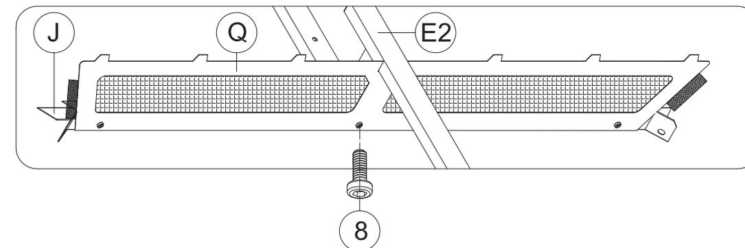
(2) Place the Assembled Part #J & #Q on Part #E2, securing with 1 Bolt #8.
