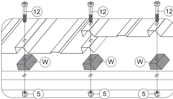
(3) Place 4 Part #W between roof panels and solidifying bars. Then secure with 4 Bolts #12 and 4 Nuts #5.
