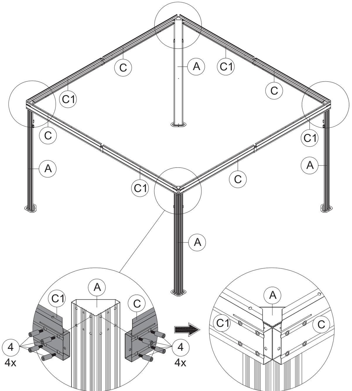
(1) Connect Part #C/C1 to Part #A with 8 Bolts #4.(From Outside)
