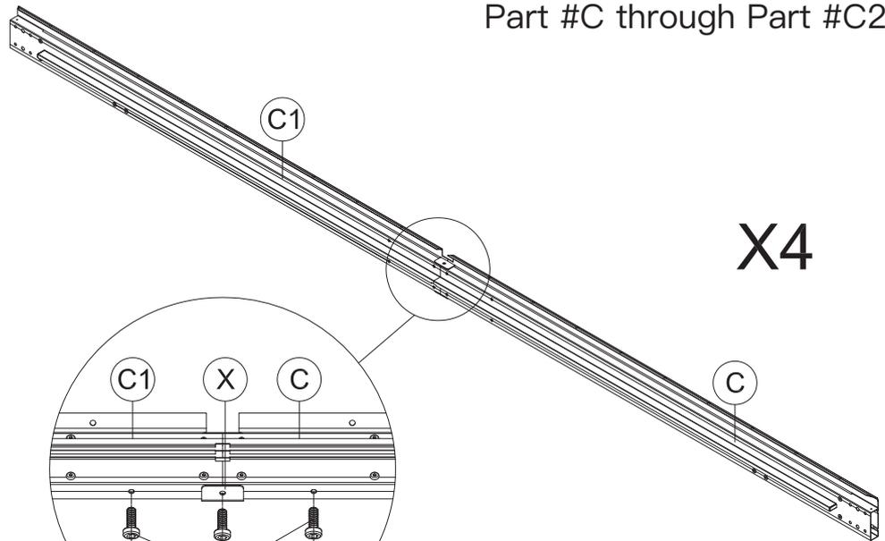
(5) Secure the bottom of Part #X and Part #C/C1 with 3 Bolts #8.
