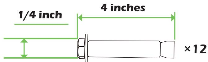
If the ground is concreted and the depth of it is over 3 inch, you can use 1/4 inch expansion bolts to mount the gazebo
