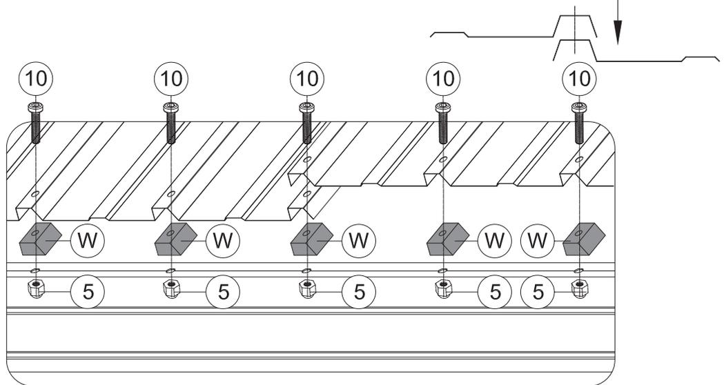
(3) Place 6 Part #W between roof panels and beams. Then secure with 6 Bolts #10 and 6 Nuts #5.
