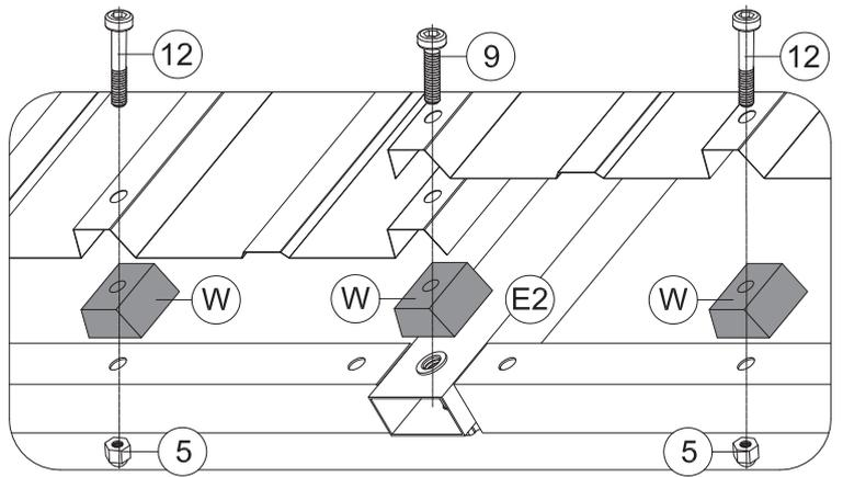
(3) Place 4 Part #W between roof panels and solidifying bars. Then secure with 4 Bolts #12 and 4 Nuts #5; Place 1 Part #W between roof panels and Part #E2. Then secure with 1 Bolt #9 and 1 Nut #5.
