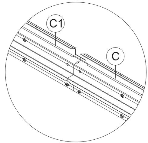
(3) Connect Part #C1 and Part #C through Part #C2.
