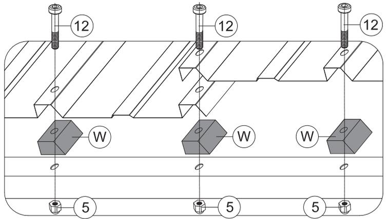
(3) Place 4 Part #W between roof panels and solidifying bars. Then secure with 4 Bolts #12 and 4 Nuts #5.
