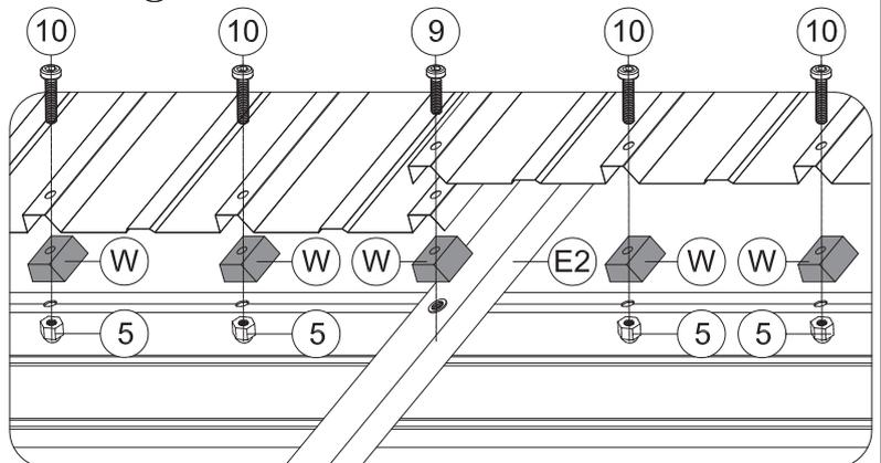
(4) Place 6 Part #W between roof panels and beams. Then secure with 6 Bolts #10 and 6 Nuts #5; Place 1 Part #W between roof panels and Part #E2. Then secure with 1 Bolt #9 and 1 Nut #5.
