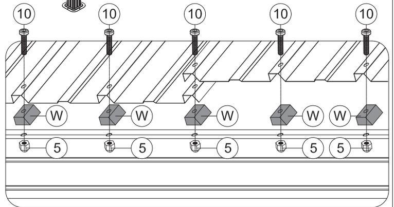
(4) Place 6 Part #W between roof panels and beams. Then secure with 6 Bolts #10 and 6 Nuts #5.
