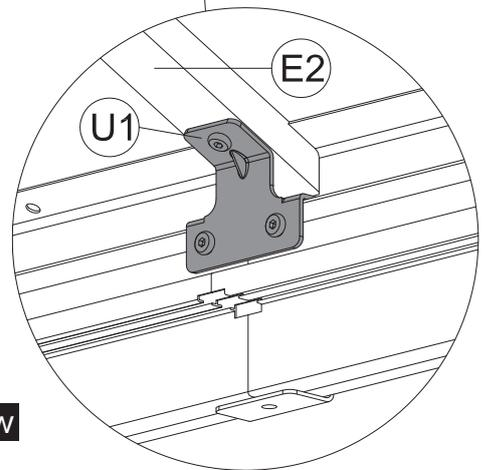
(2) Connect Part #E2 and the Assembled Beam(C&C1) with part #U1.
