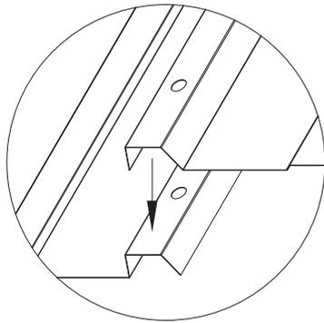
(1) Insert Part #M1 and Part #M2 into the frame.
