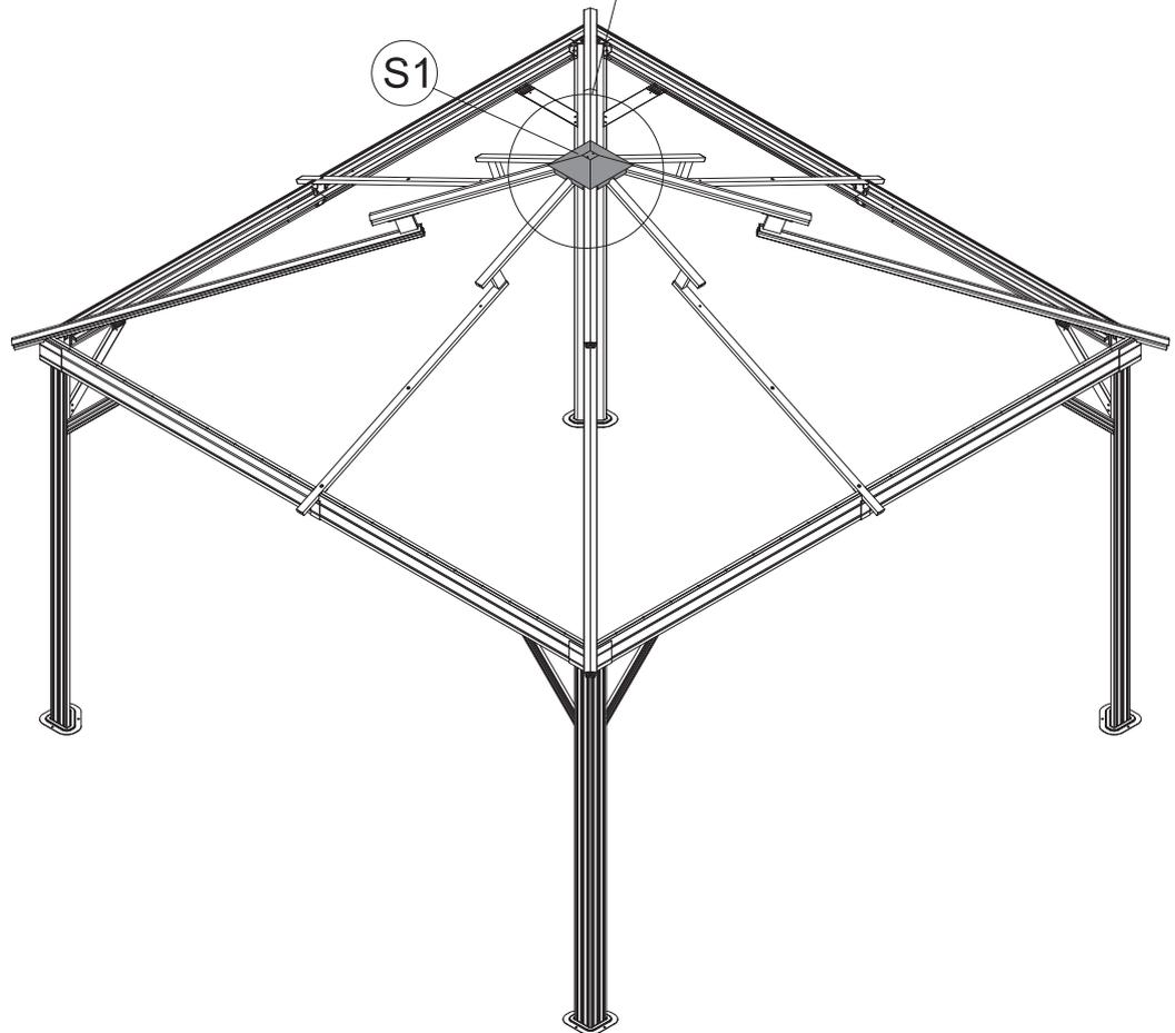
**ATTENTION:** The holes of Part #S and Part #S1 need to be aligned, on the same vertical line.
