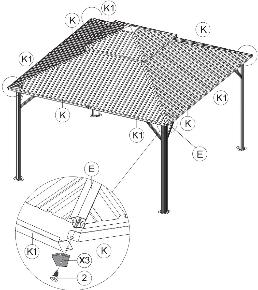
(1) Place Part #K1 and Part #K on Part #E; Put on Part #X3 and secure with Self-tapping Screw #2.
