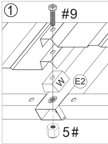
▲ Part #W should be inserted between roof panels and solidifying bar or beams, then secure with bolts and nuts.
