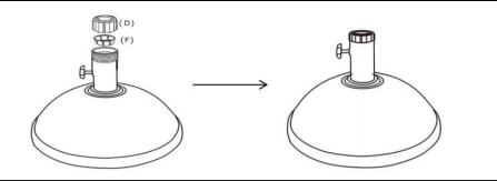
For the Umbrella pole with diameter as 48mm, use dia.48mm Adaper (F) only, insert the dia.48mm Adapter (F) into the Steel tube (B).
