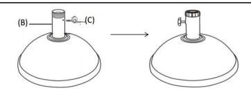
Screw Adjustable screw (C) into Support Pole (B).
