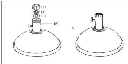
For the Umbrella pole with diameter as 38mm, use dia.38mm Adapter (E) & dia.48mm Adapter (F) added together, insert the dia.48mm Adapter (F) into the Support Pole (B) firstly, and then put the dia.38mm Adapter (E) onto the dia.48mm Adapter (F). Turn the Cap (D) onto the Support Pole (B) to hold the Adapters in place.
