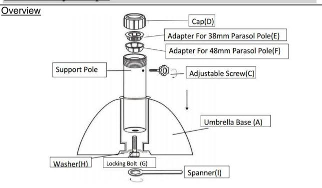
This UMBRELLA BASE as multiple parts and may require up to some 30 minutes to assemble. To give you an overview of the UMBRELLA BASE parts, the above picture is to help you put the various parts into perspective. Please read through the instructions herebelow to familiarise the parts and steps before assembly.
