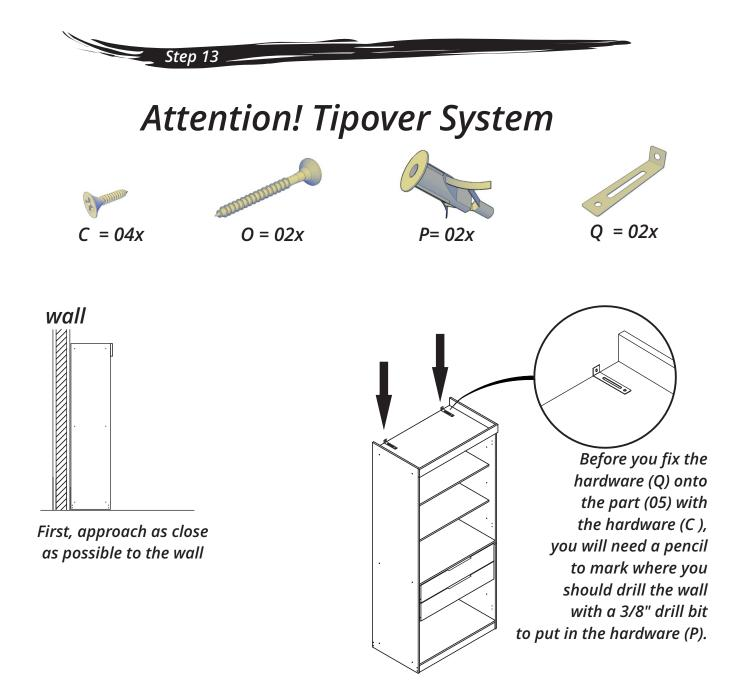
\*press the hardware wings (P) to put in the hole that you drilled in the wall.
