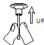
1. simply push up on the cable to raise the height of the fixture
