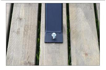
Now attach the other end of the cross brace to the underside of the table top using one of the 50mm coach screws and 2 washers, ensuring that the hole is centrally aligned across the middle slat of the table top.
