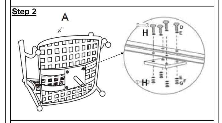
Attach the Iron Plate(B) to the undersidebase of the Chair Seat(A).
