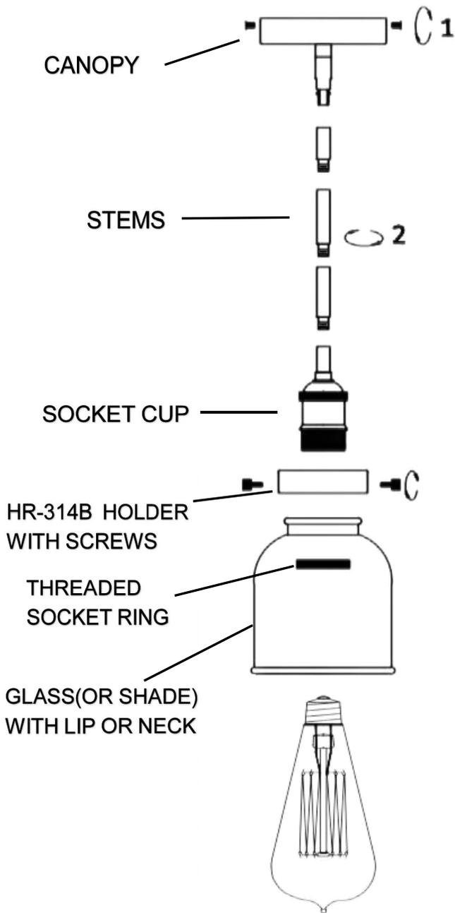
CHOOSE THE NUMBER OF STEMS NEEDED FOR THE CEILING HEIGHT THEN FEED THE WIRES THROUGH THE STEMS, THEN SCREW THE STEMS INTO THE TOP OF THE FIXTURE AND INTO THE SWIVEL ON THE CANOPY.
