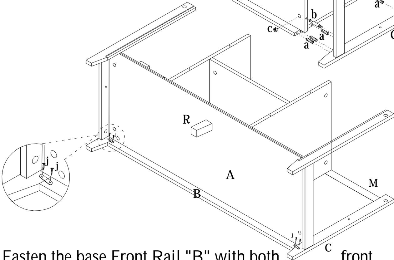
Fasten the base Front Rail "B" with both front legs "C" and "F" by flat metal bracket "j".
