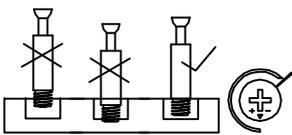
**Note: Please don't over tighten all the cam screws .Assure the cam screw just fit in the plastic threaded insert .Otherwise,the cam nut might not be able to catch the cam screws.**
