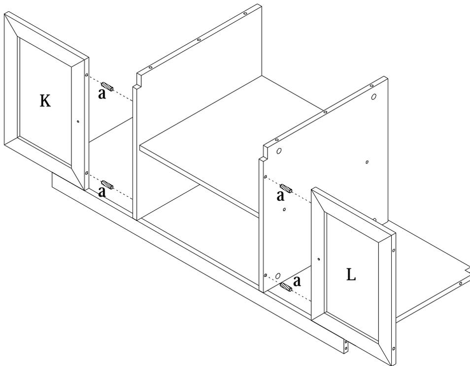
Note: Knob hole on the faux door panel is close to middle side panels.
