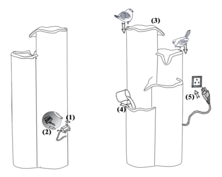
**STEP 1:**Connect the flexible tube pre-assembled inside of the fountain to the outlet of the pump.
