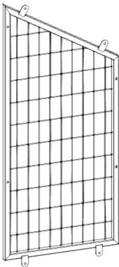
MP02 METAL PANEL - A4M02618 (x1) 1 1/16"X20 1/2"X46 15/16" (27x520x1192)
