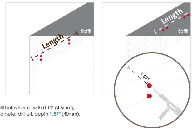
(3). Drill holes in roof with 0.19" (4.8mm), diameter drill bit, depth 1.57" (40mm).
