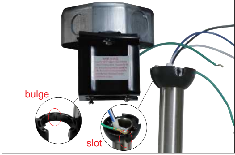
Step 11 Hang the fan on the hanging bracket and align the slot on the downrod with the bulge on the hanging bracket.
