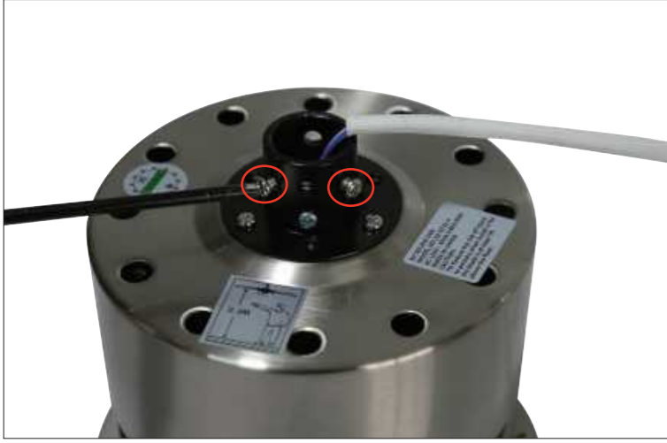
Step 4 Loosen the 2 screws of the coupler.
