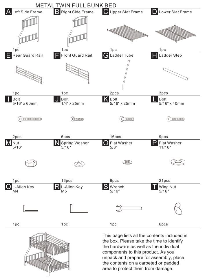
Attach Left & Right Side Frame (A & B) to Upper & Lower Slat Frame (C & D) using Bolt (K), Spring Washer (N) and Flat Washer (P) with L-Allen Key (R).
