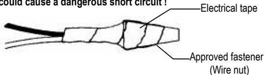
6. Connect the black fixture wires to the black wire in the outlet box. Fasten the joined wires as in step 5.
