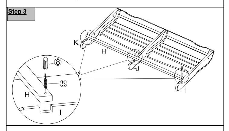
Position Back Support (H) on to the tract of Long Legs (I), (J), (K) using 3 Screws(5) and Screwdriver (8).
