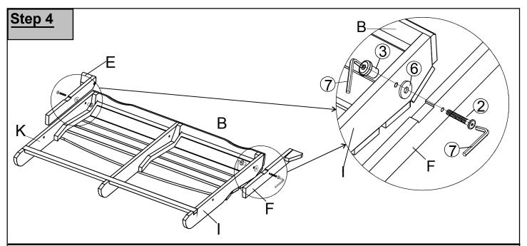
Attach Short Left Leg (E) and Short Right Leg (F) onto Long Left Leg (K) and Long Right Leg (I) using 2 Bolt (2), Plastic Washer (6) and Sleeve Nut (3) with Allen Keys (7).
