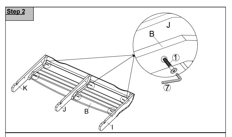
Place the Seat Panel(B) onto a clean, non-marring surface Position Long Legs (I), (J), (K) onto the Seat Panel(B) and attach using 6 Screws(1) and Allen Key (7).
