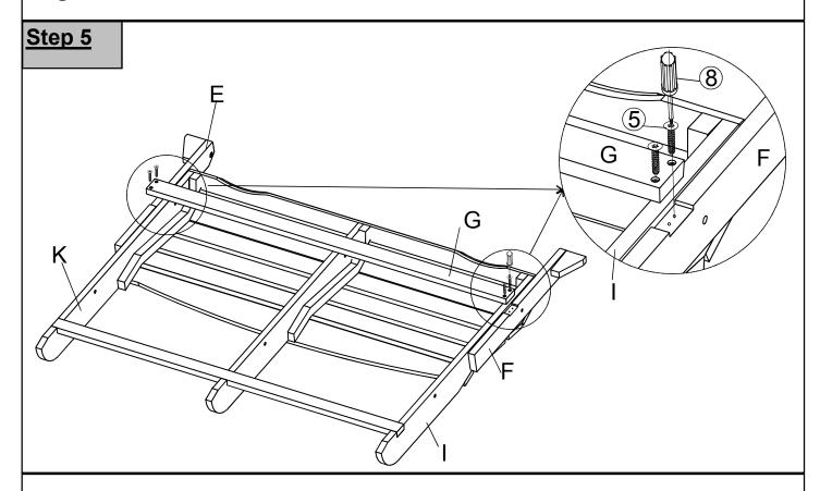
Position Front Support (G) onto the tract of Short Legs (E), (F) using 4 Screws (5) and Screwdriver (8).
