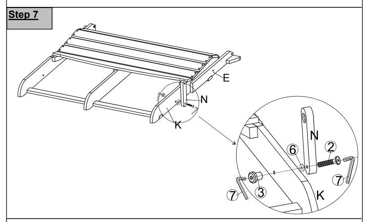
Reverse Seat panel in Step 5 in the position as picture above Attach Folding Support Bars (N) to Long Left Leg (K) using Bolt (2), Plastic Washer (6), Sleeve Nut (3) and Allen Key (7).
