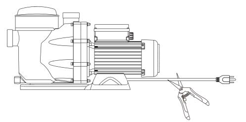
2. Peel off the black cable skin to reveal the 3 wires inside, strip each cable by 2/3 inch with a wire stripper, then strip the insulation to reveal 1/5 inch copper wire. Prepare the wire extension of the pump and repeat the above steps.
