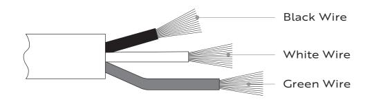
Insert the stripped wires into the butt connectors in the wire pigtail from the pump. Firmly crimp each splice with crimping plier to tightly hold the wires in place. Attention: Please ensure correct matching when wiring an extension cable.
