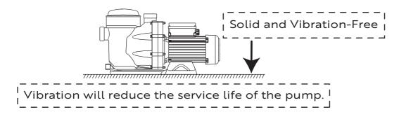
2. Fill the pump with water before starting. Do not run pump dry. Water acts as a coolant and lubricant for the mechanical shaft seal. Running pump dry may damage seals, causing leakage, flooding, and void warranty.
