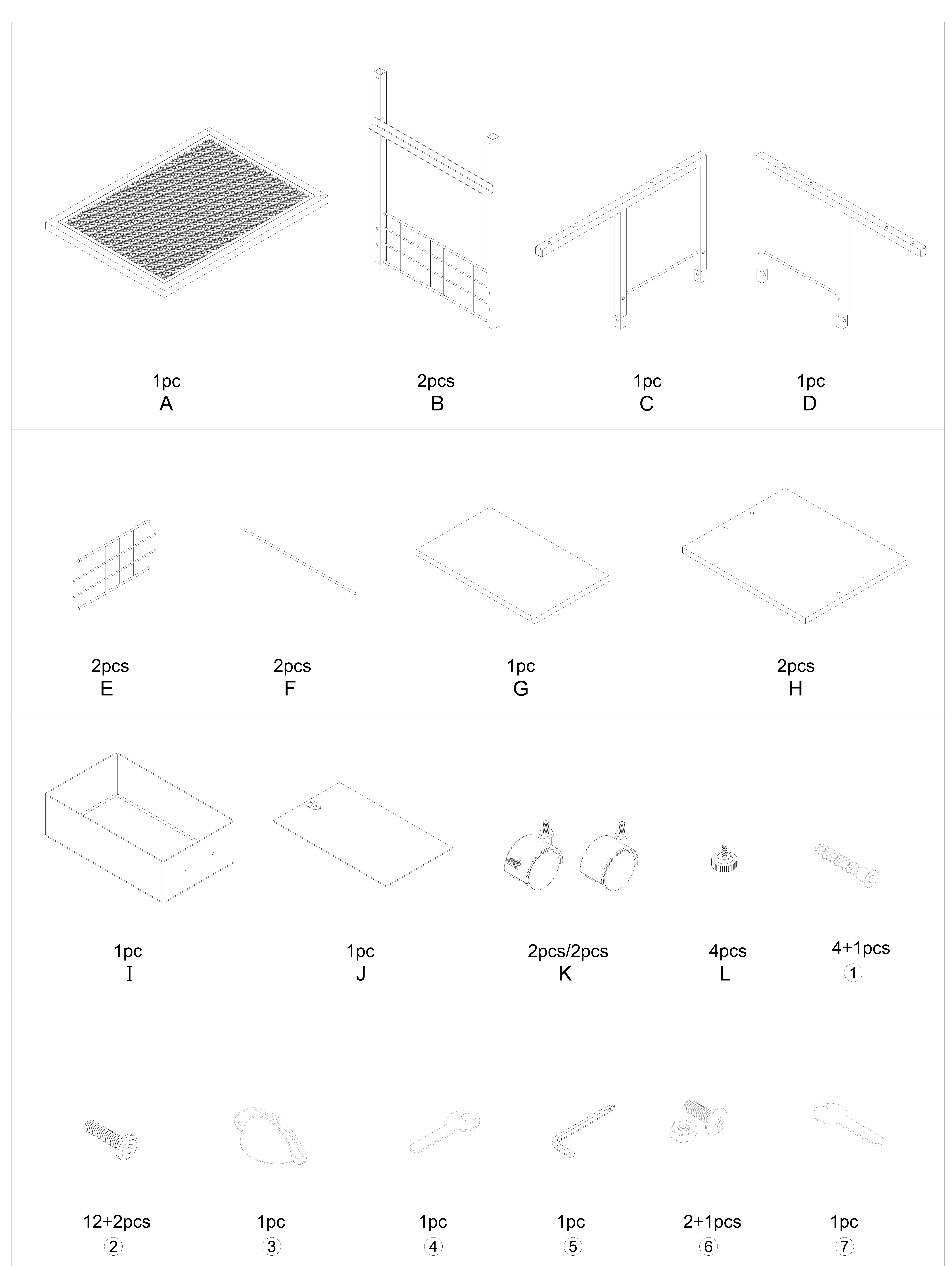
1. Use Screw ② to attach one Component B to the front of Component A.(The front of Component A has 4 holes).
