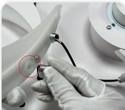
4 Tighten the nipple screw
