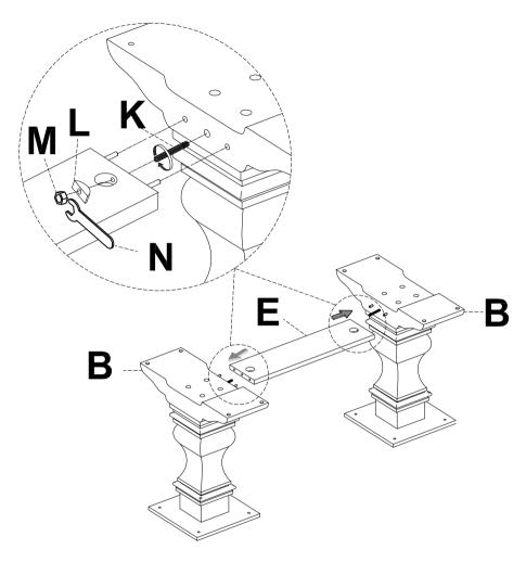
STEP 3:Align Table strecher (E) to the Table base (B), then secure by using threaded pins (K) with half moon (L) and hex nut (M).
