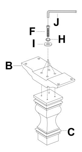
**STEP 1:**Align Table base (B) to the Table pillar (C), then secure by using bolts (F) with washers (H,I).
