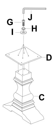
**STEP 2:**Align Table Connection plate (D) to the Table pillar (C), then secure by using bolts (G) with washers (H,I).
