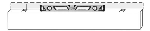
Step 4: Take the shelf off the wall and place it aside. Using a level that reaches both of your marks, (you can use a yard stick and rest your level on top of it if your level is not long enough) verify that your indicator marks are level. With the level still in place, draw a horizontal mark that connects to the marks you already made in Step 3.
