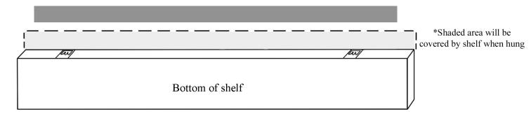
Step 3: With the help of a partner, place a level on the back of the shelf and level it. Make 2 small vertical marks that line up with the inner edge of each bracket. Be sure your marks line up with the edge of the brackets, not the edges of the cutouts.
