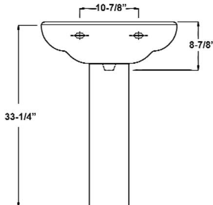
Dimensions of fixture are nominal and may vary within the range of tolerances established by ASME Standard A112.19.2-2013. Dimensions and specifications subject to change without notice.
