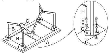
With assistance from your adult partners, turn the Cocktail Table right way up. Adjust the Pre-installed Levelers on the bottom of Leg (B) until the Cocktail Table is level with the ground.
