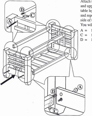
Attach the newspaper rack (P3) and upper rail (P4) to the table leg (P2). Complete one side first and repeat the same for the other side of table leg (P2).
