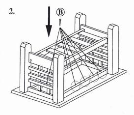
Place the table top upside down on a non-abrasive surface. Attach the table top to the upper rail. You will need to use hardware:
