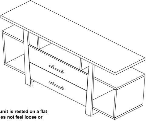
Make sure the unit is rested on a flat surface and does not feel loose or wobbly. If it does, double check all bolts/screws are secured and properly tightened.
