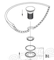
Insert the drain top into the vessel. Install thick rubber washer, 2 O-rings and mounting ring in turn.
