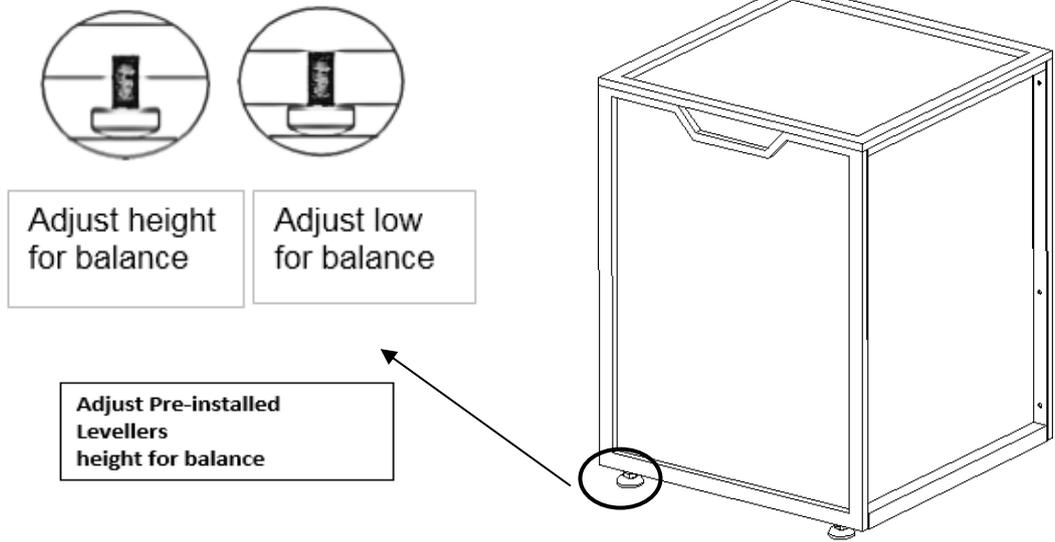
If the Tank Holder wobbles, adjust the Pre-installed Levellers at the bottom of the Panel (A) & Panel(B) until the Tank Holder is level.
