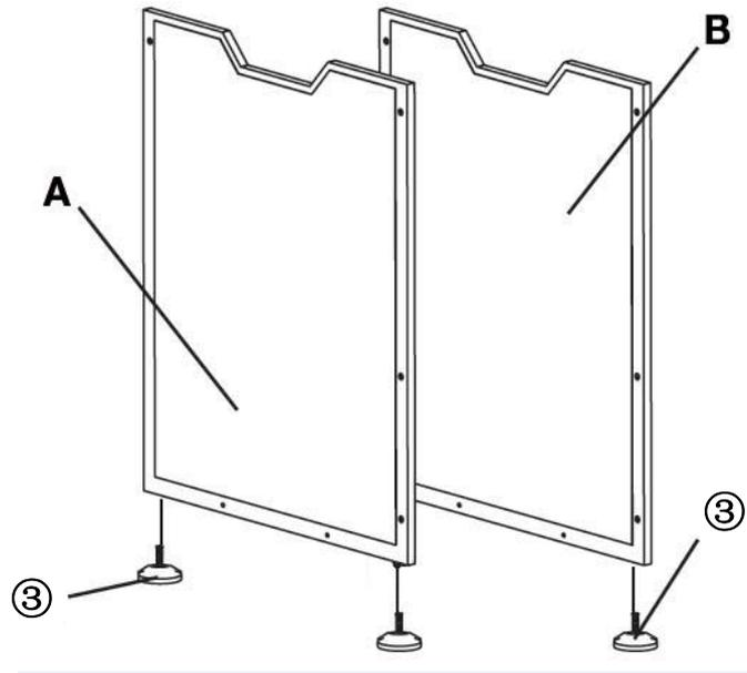
Assemble the 4 Leveller (③) to the bottom of the Front Panel (A) and Back Panel (B).
