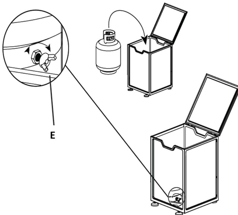
Place a 20 lb. Propane Gas Tank (not included) on top of Stand (E). Turn the Preassembled Wing Screw on the Stand (E) clockwise to secure the Gas Propane Tank.
