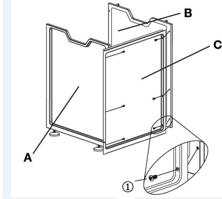
Attach the Side Panel (C) to the Front Panel (A) and Back Panel (B) using Screw(①), with Screwdriver(④).
