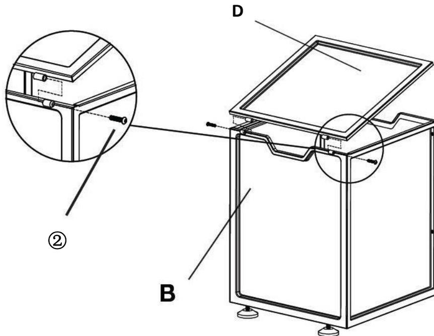
Attach the Top Panel (D) to the Back Panel (B) using M6 Screws (②) with Screwdriver(④).
