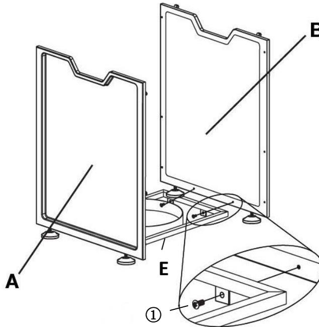
Attach the Front Panel (A) and the Back Panel(B) to the Stand (E) using M5 Screw (①), with Screwdriver(④).
