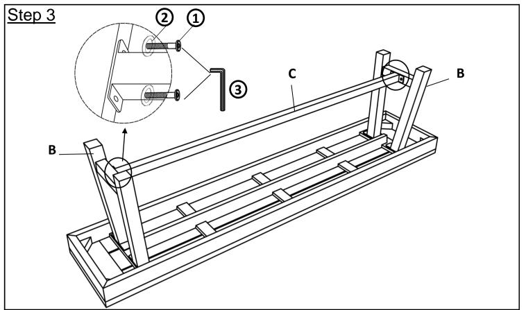
Attach Support Bar(C) to Iron Legs(B) using Bolts((1)), and Washers((2)) with Allen Key((3)) as pictured above.
