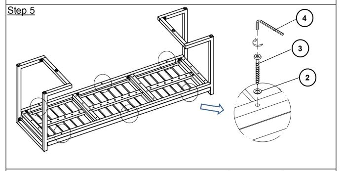
Attach the Iron Leg Frames(B) to the Bench Seat Panel(A) using Screws(3) and Washers(2) with Allen Key(4).
