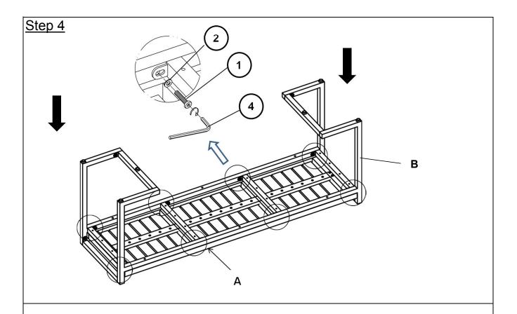
Position the Bench Seat Panel(A) facedown on a clean, non-marring surface. Align the Iron Leg Frames(B) to Bench Seat Panel(A) as pictured. Attach Bench Seat Panel(A) to Iron Leg Frames(B) using Bolts(1), and Washers(2) with Allen Key(4). **Do not fully tighten the Bolts.**
