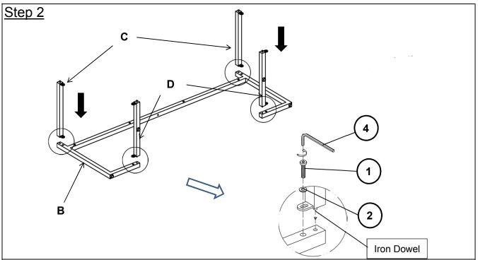
Position the Iron Leg Frame(B) facedown on a clean, non-marring surface.
