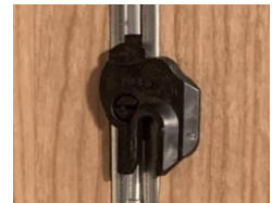
Figure 5. Actuator in the closed position
