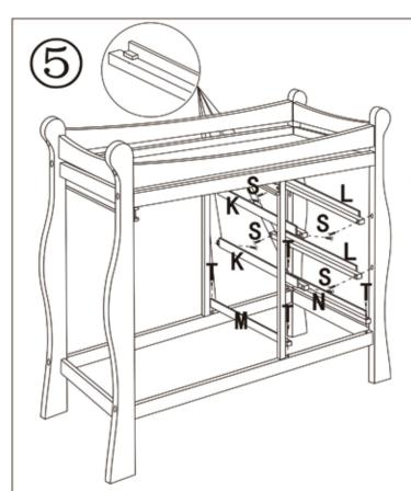
ATTACH THE TOP/MIDDLE BASKET TRACKS (PARTS K AND L) TO THE RIGHT SIDE PANEL (PART B) AND VERTICAL POSTS (PART F) USING PART S BOLTS. ATTACH THE BOTTOM BASKET TRACKS (PARTS M AND N) TO THE BOTTOM RAILS (PARTS E) USING PART T SCREWS.
