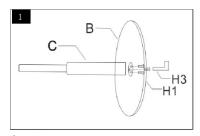
Step 1 Align the gas lift (C) onto the base as pictured. Use allen key "H3" to lock the 3 screws "H1".
