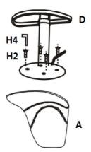
Step 3 Align the column (D) onto middle of the frame as pictured. Use allen key "H4" to lock the 4 screws "H2".
