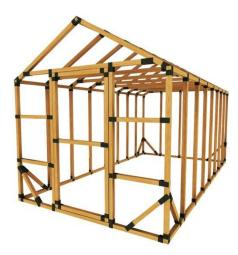
Note: When assembling your structure make sure you put a screw in each hole in each bracket to make sure your structure is rigid and solid when completed.
